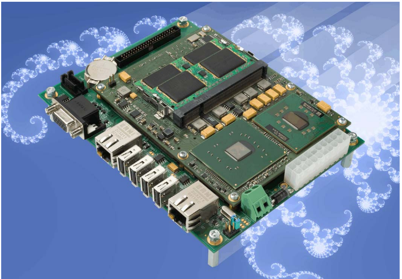
XV2 COM Express Carrier Board with XB1 COM Express CPU Module
